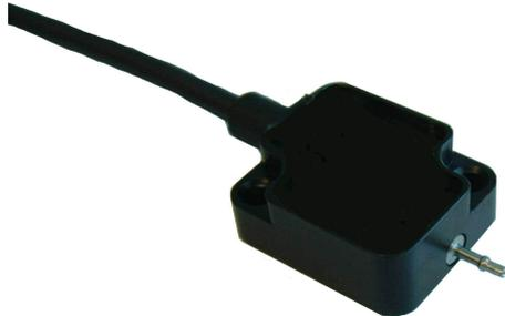
The gain, offset and thermal drift of the pressure sensor is digitally compensated to minimise errors and to create a single-ended, amplified output in the 0.5 to 4.5 Volt range. The output voltage changes with the absolute pressure applied to the pressure port
